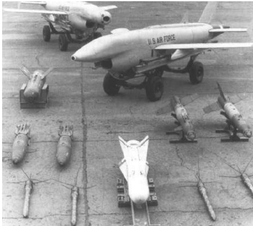
Figure 1.3: BQM-34 Firebee series with the ammunition kit. The white missile located at the center of the picture is an AGM-65 Maverick, successfully launched in tests in the early 1970s. Picture by Bud Wolford, retrieved from [20].
