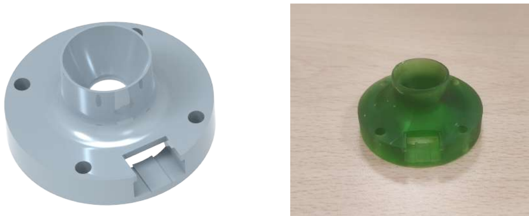
Figure 2.13: Nozzle design, and manufactured version with resin.
