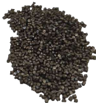
Figure 2.7: Propellant used for the gas generator
