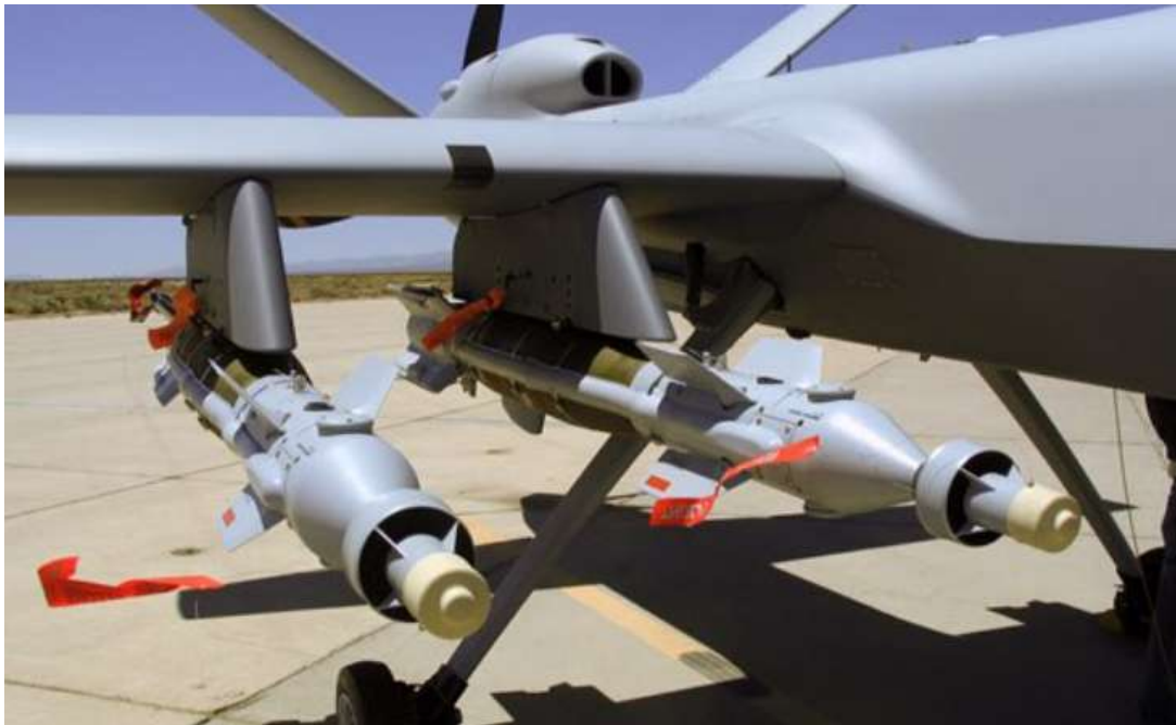
Figure 1.5: Closer view to the inboard and outboard hardpoints of the Reaper, carrying the before mentioned GBU-12 Paveway II laser guided bombs of 295 kg. Developed in the 1970s, it carries a general purpose warhead.
