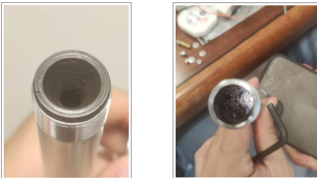
Figure 4.23: Nozzle and casing after test 3.
