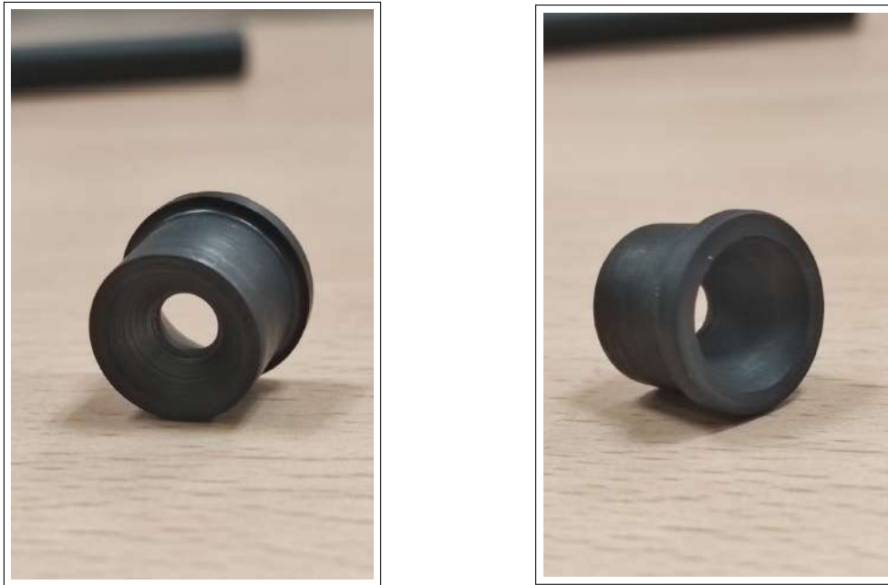
Figure 3.15: Views of the manufactured graphite nozzle.
