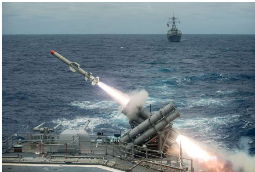
Figure 2.2: Harpoon missile launched from the USS Shiloh, September 15, 2014. The missile is deployed from one of the tubes of the multiple-tube launcher system, with the ignition of the launch motor. Please notice the important rocket plume, blast, and exhaust gases that the launch motor produces. Image: US Navy/Mass Communication Specialist 3rd Class Kevin V. Cunningham.
