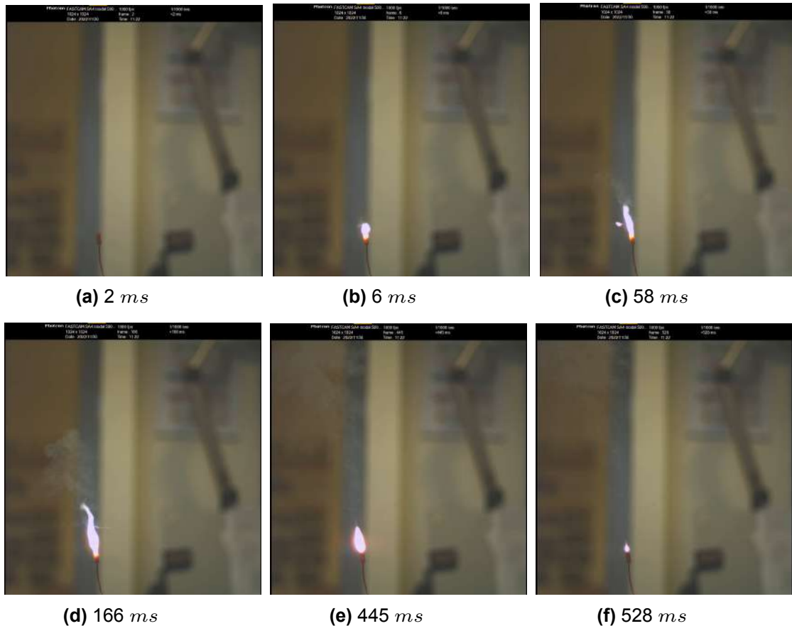
Figure 2.6: Phases of electric match ignition after triggering. Stage (b) shows an already ignited match. At stage (d), the flame created by the electric match reaches its full extension. The response time, after the triggering of the launch signal, and before ignition, is around 4 ms .
