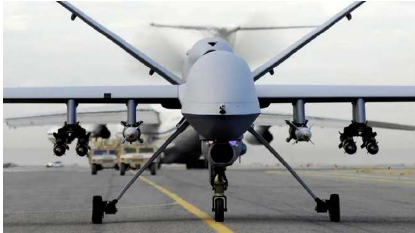
Figure 1.4: This MQ-9 Reaper model carries two GBU-12 Paveway II laser guided bombs in the inboard stations, and 4 Hellfire missiles in the outboard stations, while taxiing in an Afghanistan Runway. U.S. Air Force photo/Staff Sgt. Brian Ferguson.
