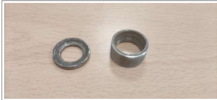
Figure 4.18: Broken Bulkhead of test 2.
